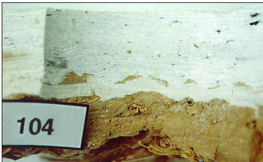
Figure 3. Core ( \varnothing 5 cm) of restaured plaster - bond between gypsum backfill mortar and loam
