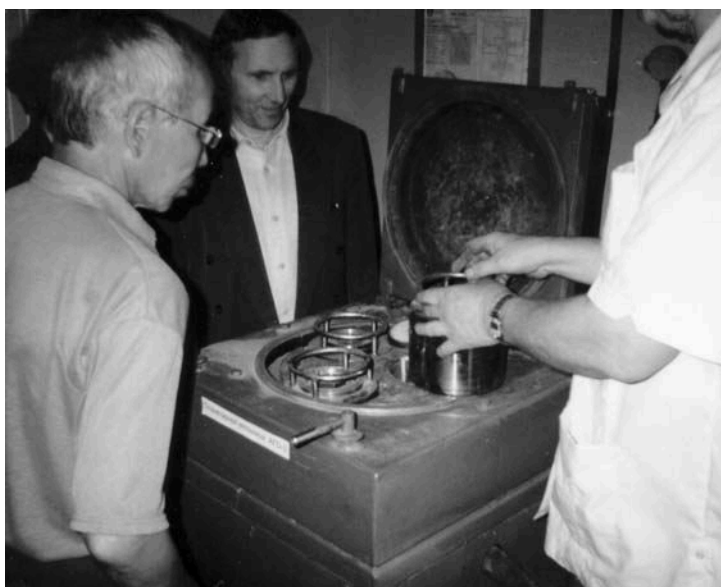
Figure 5. The laboratory activator mill AGO-3
