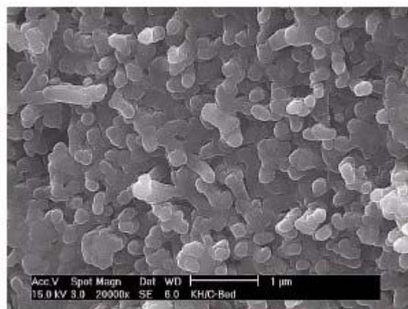
Figure 5. The same sample as in Figure 4, but with an approximately 30 nm thick layer of carbon for imaging in conventional SEM. The morphology of the C-S-H phases are changed drastically by the thermal stressing during the coating process and by the vapour-deposited layer.
