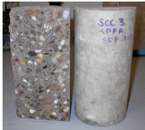
Figure 5. Mix SPFA1 following a slump flow test and the aggregate distribution in a hardened sample
