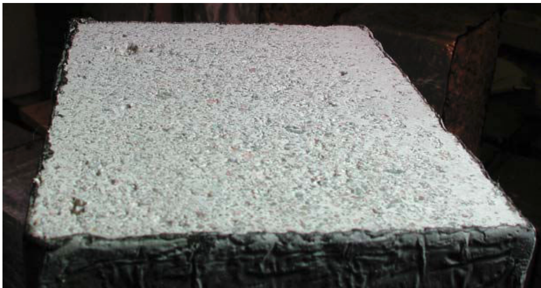
Figure 11. Surface scaling of 200 \text{ g/m}^2 of a CIF test specimen after 56 freeze-thaw cycles.
