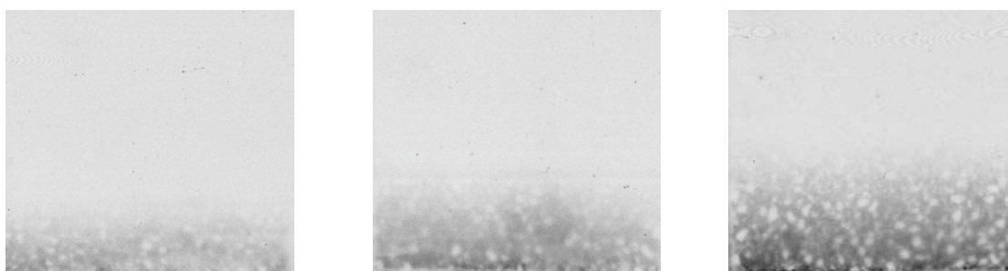
Figure 1. Autoradiography of cement mortar after 14, 33 and 55 days in labelled solution
