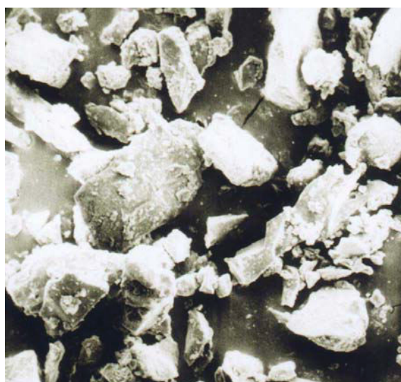
Figure 3. Structure of HAP x 400
