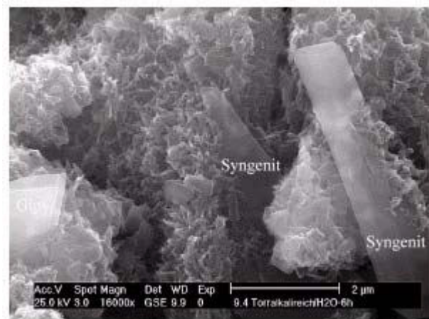
Figure 11b. Microstructure after 6 hours hydration time [high potassium content]: syngenite is starting to dissolve with formation of secondary gypsum (left).
