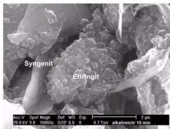
Figure 9b. Microstructure after 10 min hydration time [high potassium content]: Ettringite with the same morphology as cement with low arcanite content. Formation of syngenite (lath-shaped crystals).
