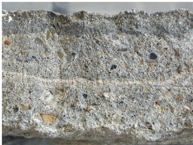
Figure 5. Sample of shotcrete lining of “Koblenz” railway tunnel showing several distinct layers parallel to the support (bottom) due to irregular accumulations of sand, aggregate, paste and air voids.
