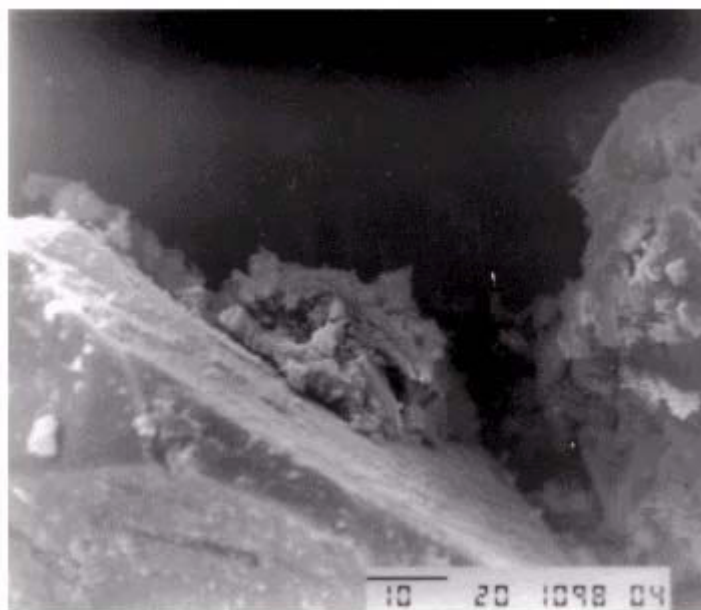
Figure 2. Slag grains with coating surface of hydration/carbonation and probably sulphate products
