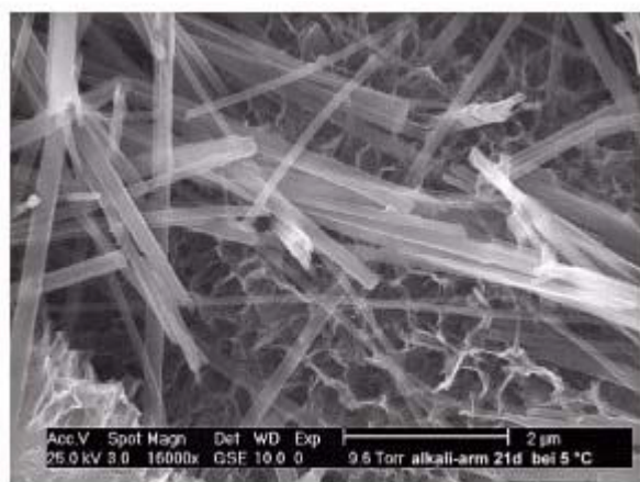
Figure 19a. Microstructure after 21 days hydration time at the temperature of 5 °C: very long prismatic ettringite (up to 4 \mu m ).
