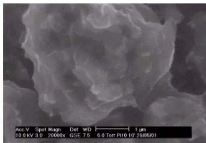
Figure 8. ESEM-FEG image of a clinker ground with 0.5% of PCAE + 0.5% of H_2O and pasted with water ( w/c = 0.4).
