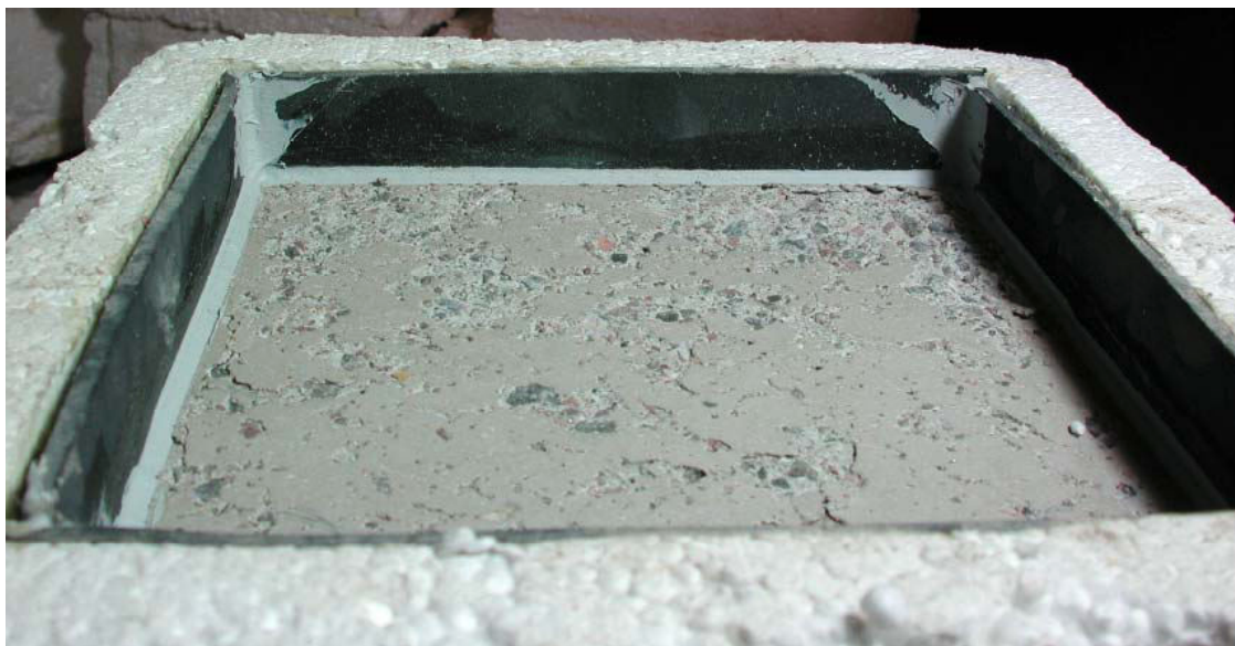
Figure 12. Surface scaling of 550 \text{ g/m}^2 of a slab test specimen after 56 freeze-thaw cycles.
