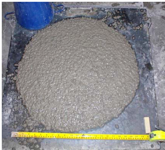
Figure 5. Mix SPFA1 following a slump flow test and the aggregate distribution in a hardened sample
