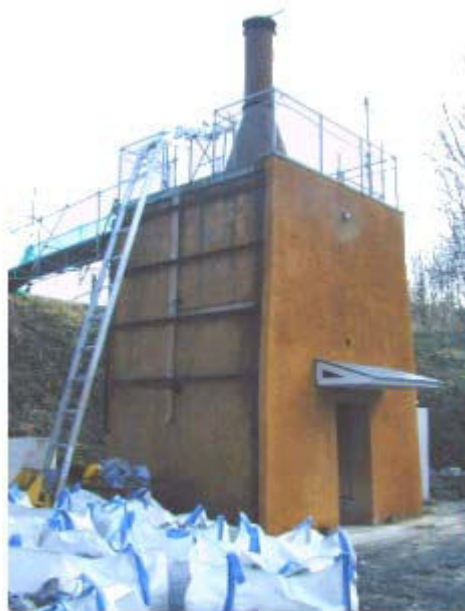
Figure 3. General side view, showing; mechanical hoist for top loading ELK, sloping front façade and restraining bars and end points of thermocouples arranged vertically on side next to hoist.
