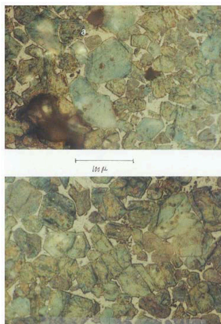
Figure 3. Optical micrograph representative of microstructures of the Star clinkers
