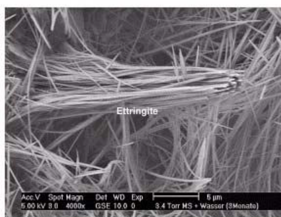
Figure 21b. Storage of monosulfate in water at 22 °C: formation of aggregates of parallel-grown ettringite crystals.
