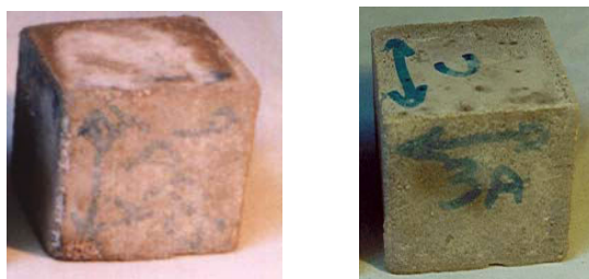
Figure 6. OPC and AAS mortars after 180 days of exposition to Sulphates
