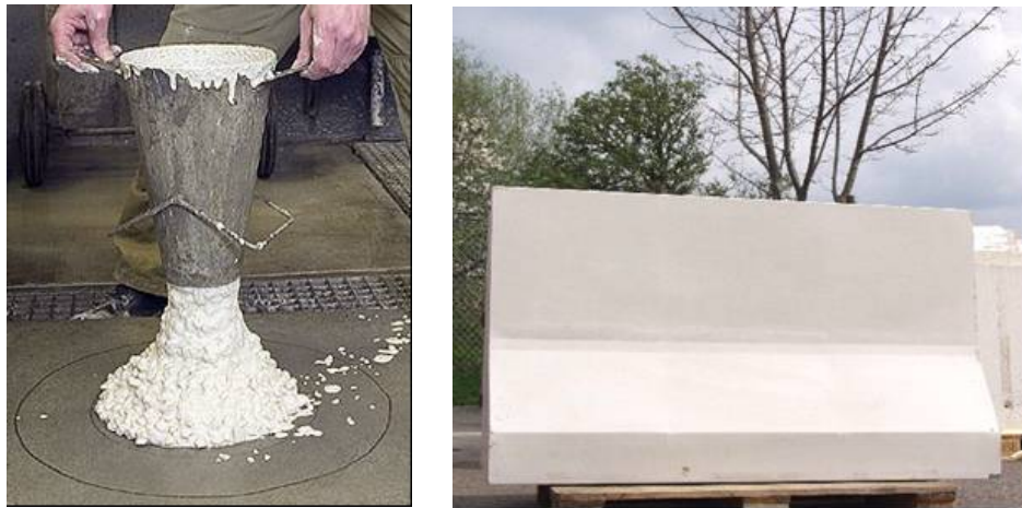
Figure 2 - Left: White SCC slump flow test. Right: White SCC provides flawless surfaces.
