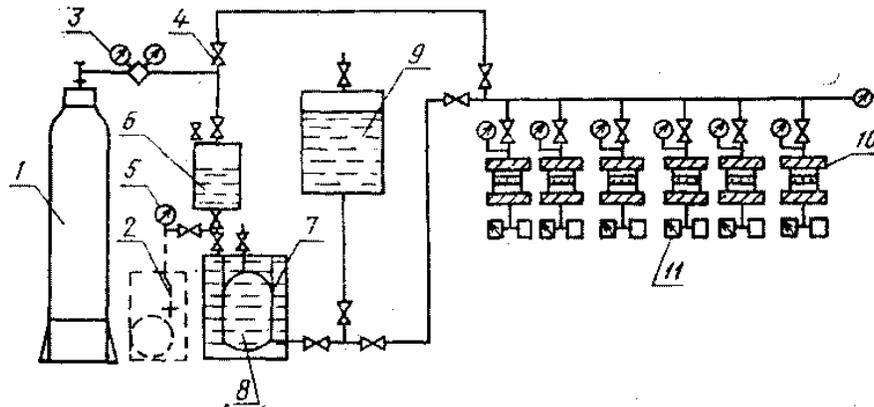
Fig. 8. Thematic diagram of the installation for testing specimens for waterproofness.
