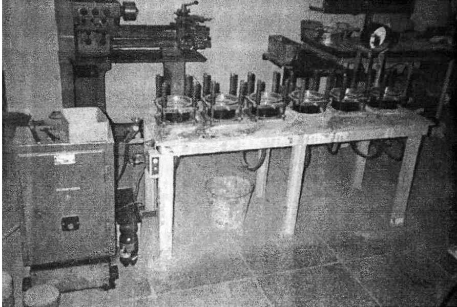
Fig. 7. The installation for testing specimens for water sorptivity
