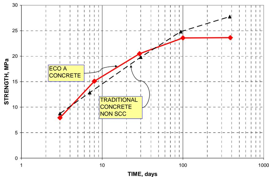
The EcoA and TRAD concretes are similar in strength until an age in the range 30-50 days. After this time the TRAD concrete, that contains significantly more Portland cement, continues to gain strength.
