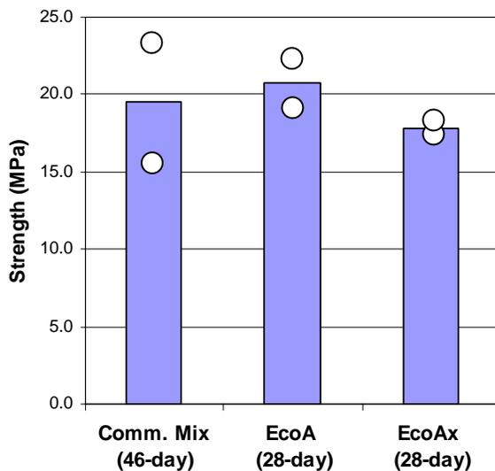
Figure 6. Average compressive strengths from 200 mm concrete cores (white circles = individual core strengths)
