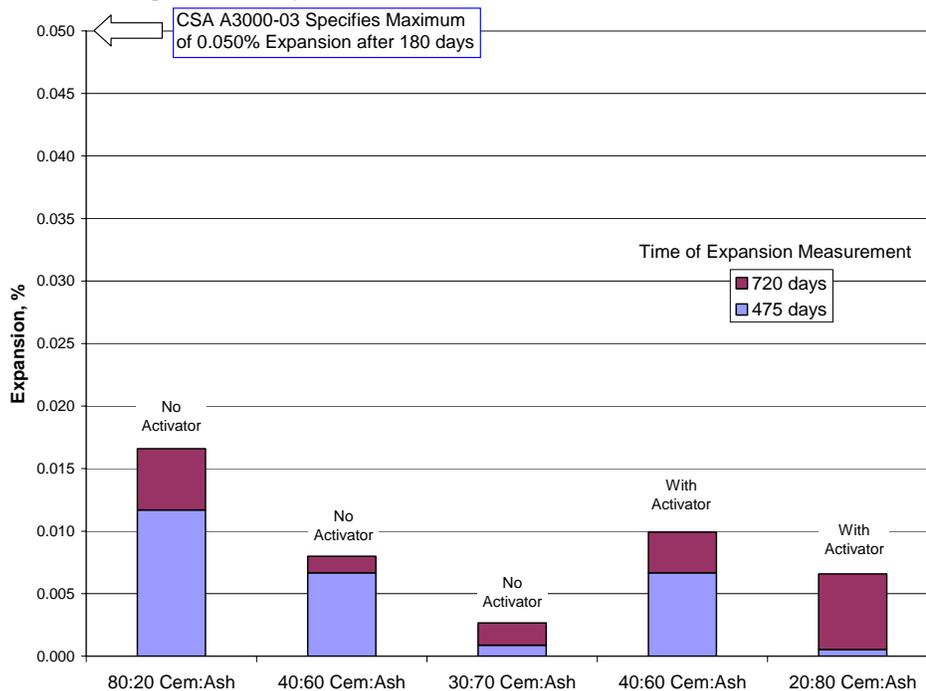
Expansions even after 720 days for all bars are much less than the 0.050% maximum allowed by CSA at 180 days for a sulphate-resistant cement. The benefits of using high proportions of fly ash is clearly shown. The addition of the activator appears to produce a slight increase in expansions, but expansions are still well below the allowable.
