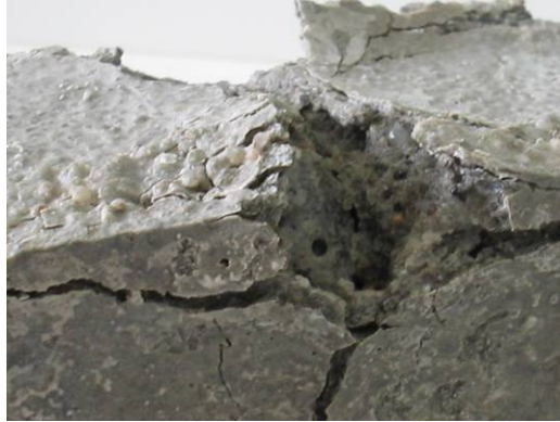
Fig. 14. The samples of CL2 cement mortar (sulphate solution, 5°C, 720 days).
