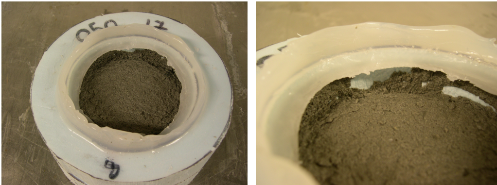
Figure 4: Degradation of the mixture prepared at a W/B 0.55 and 0% Air after 17 cycles
