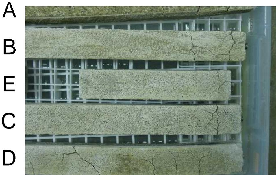
Figure 4. Mortar bars stored in 92% RH showing typical local expansion resulting in cracking.
