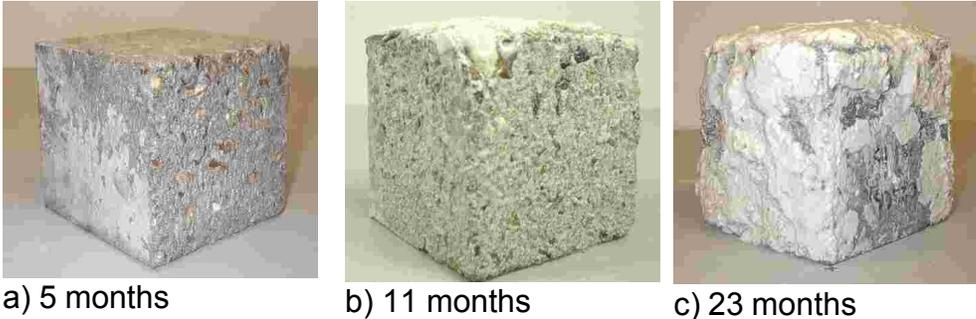
Fig. 3 OPC with siliceous aggregate in DS-3 solution for 5, 11 and 23 months
