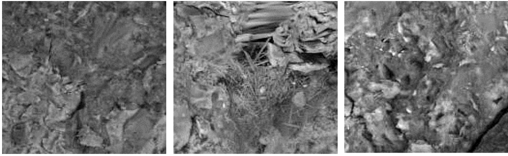
Fig. 1. Microscopic pictures of the mortars stored in comparative water environment – the differences in the structure are visible: 1 – mortar made from Portland cement CEM I 42,5, 2 – mortar made from cement CEM I 42,5 MSR NA, 3 – mortar made from cement CEM I 42,5 HSR NA
