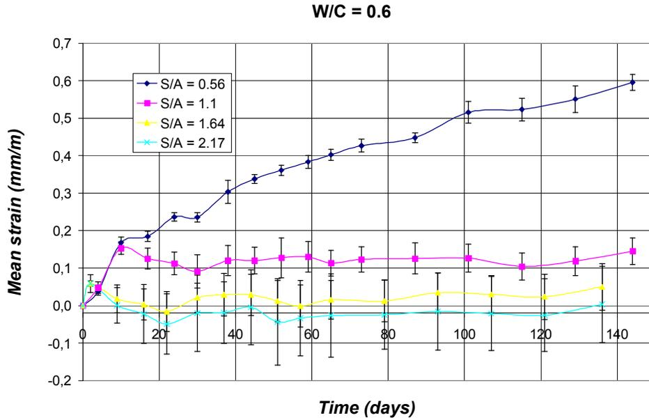
Figure 4: Expansion evolution for concrete formula at  $W/C = 0.6$
