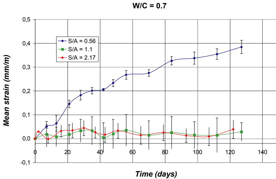
Figure 5: Expansion evolution for concrete formula at  $W/C = 0.7$
