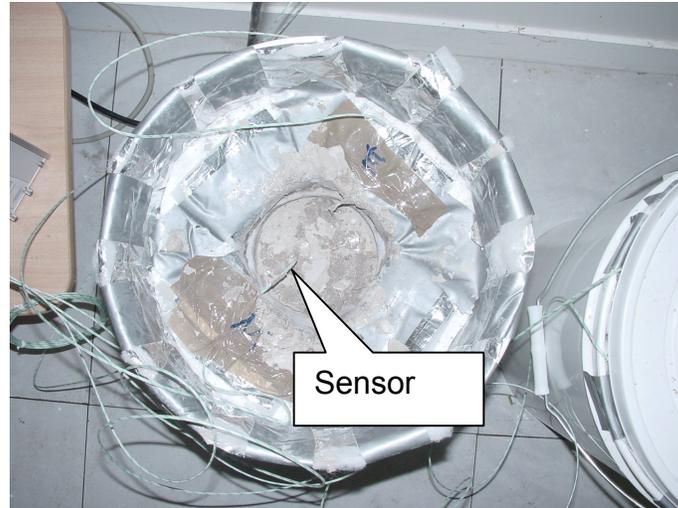
*Figure 3: Calorimeter for exothermal test*
