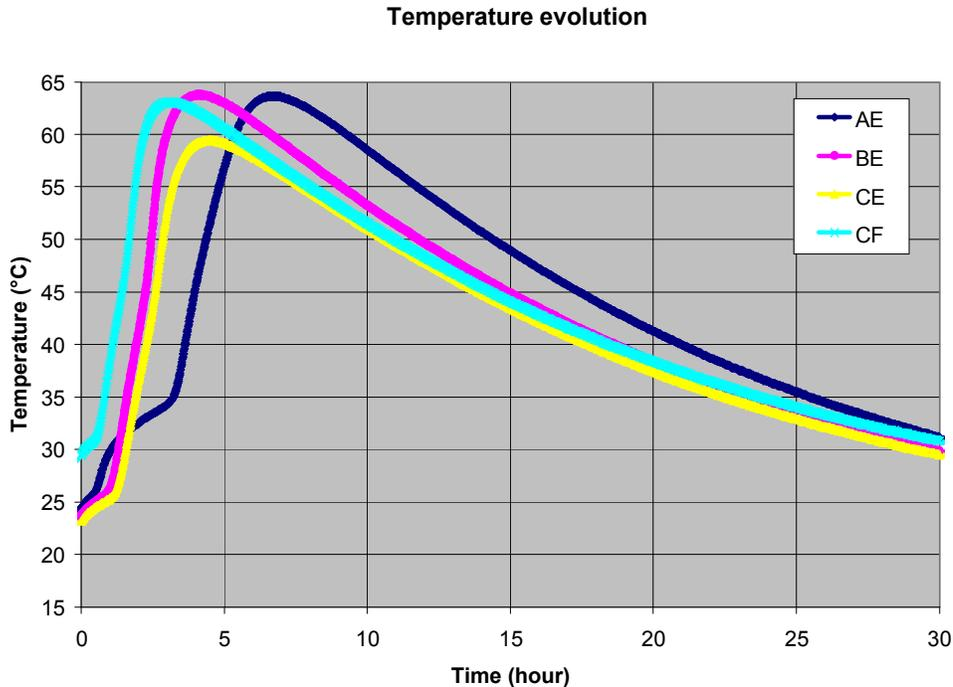
*Figure 6: Temperature evolution during the hardening of concrete.*
