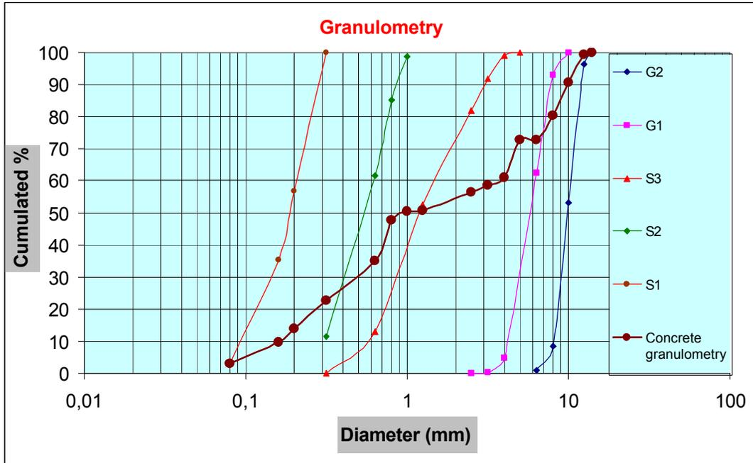
Figure 1: Granulometry of aggregates and concrete
