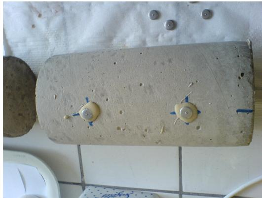
Figure 2: Jointing the studs on the specimen
