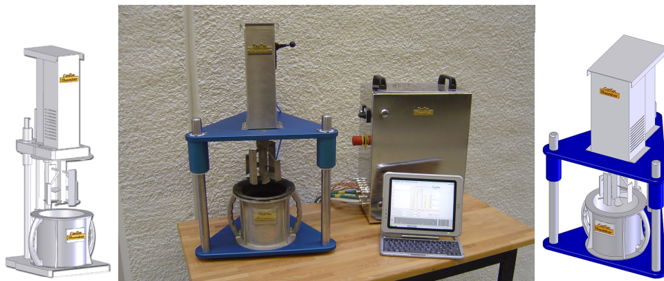
Fig. 1. The Rheomixer including 10” Tablet PC for data processing.
