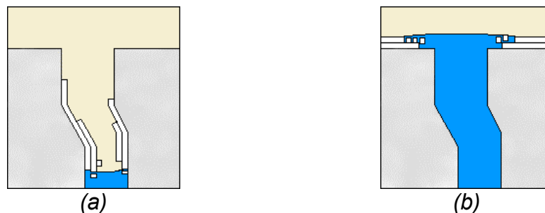
Fig. 2: Efflorescences: influence of climatic conditions.
