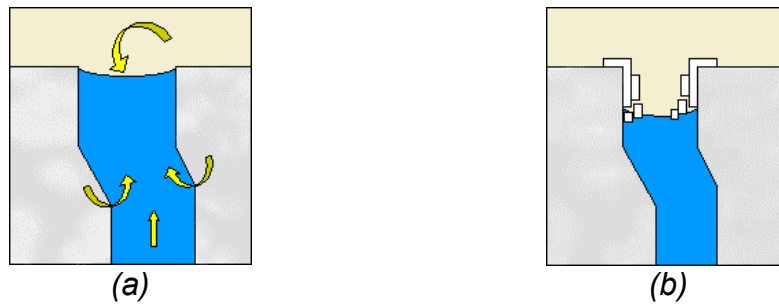
Fig. 1: Mechanism of appearance of efflorescences [2].
