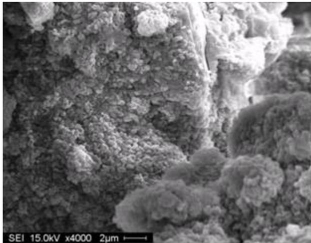
(b) Carbonated cement paste in flue gas
