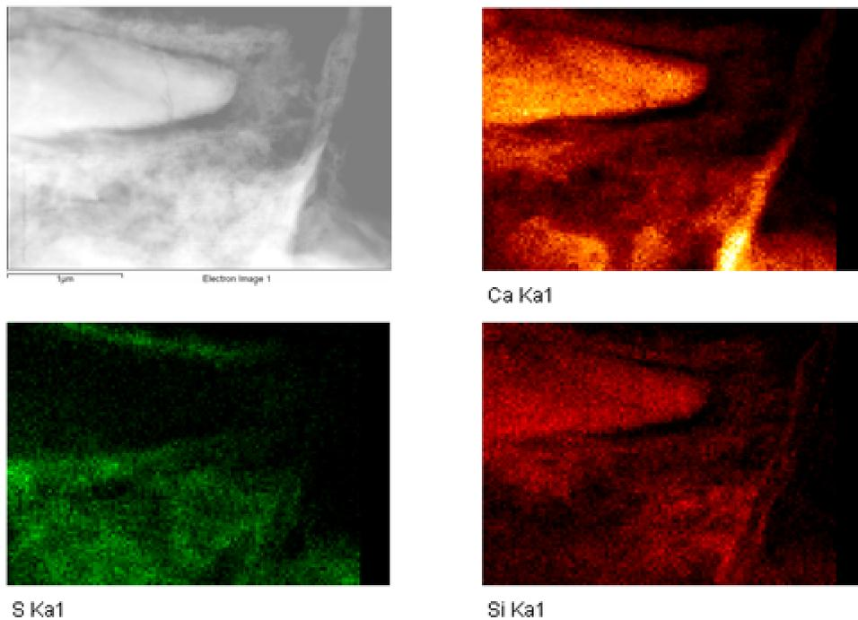
**Figure 7.** EDS chemical mapping - The S Kα1 map clearly shows the large amounts of sulfur present in C-S-H around the reacting grain
