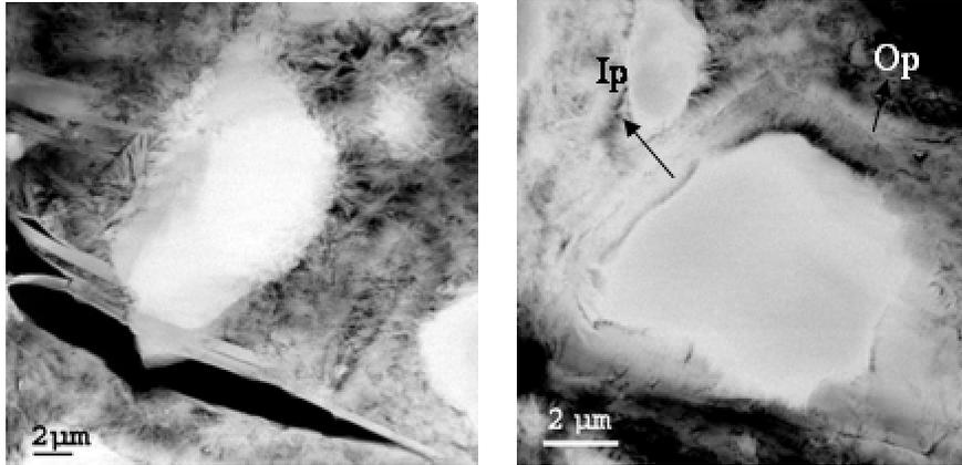
**Figure 5.** 48hrs – densification of the cementitious matrix / filling of the gaps with densifying inner product
