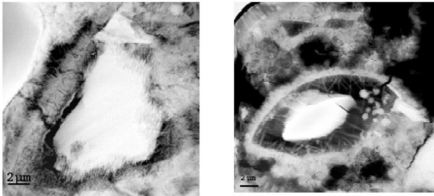
**Figure 4.** 24hrs - left : continuum between reacting alite grain and precipitating C-S-H / right : growth of ettringite needles from the shell towards the grain
