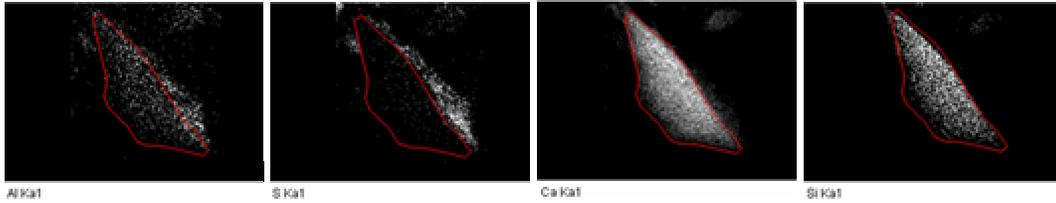
**Figure 1.** 2 hours of hydration - totally unreacted cement grains (left) and beginning of surface hydration (right) with corresponding EDS mapping
