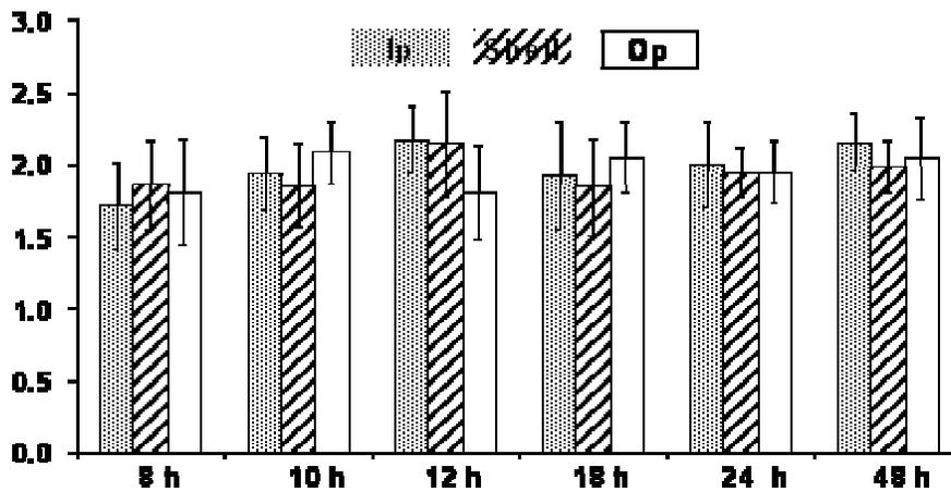
**Figure 6.** Analyses of Ca/Si ratio of product in shell, inside shell (Ip) and outside shell (Op) at different hydration times.
