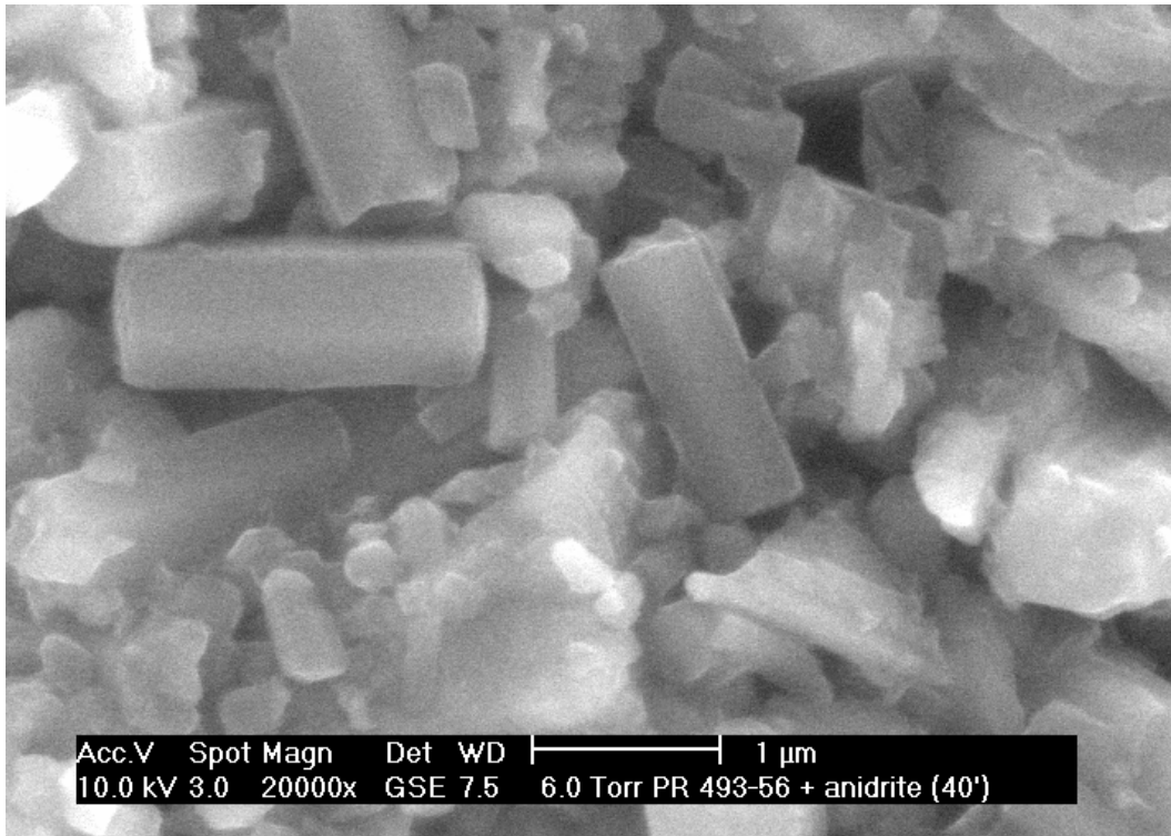
Fig. 10 ESEM micrograph of Panhd after 40 minutes of hydration (unit length 1 \mu m)
