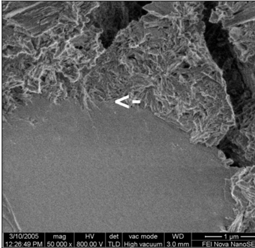
Fig. 11: C_3S grain with hydration rim: low voltage mode, U_0 = 800 V in high vacuum, partial charge build-up, loss of depth of focus (see arrow)
