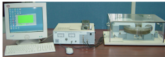
Fig.2 Photo of a non contact resistivity meter
