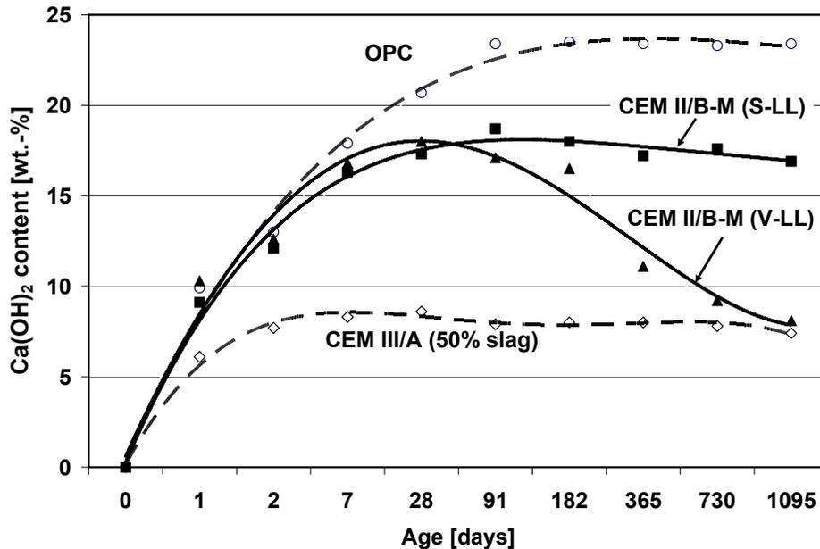
**Figure 2:** Development of Ca(OH)<sub>2</sub> in cement paste (mortar, w/c = 0.60; cured at 20°C under water until testing)
