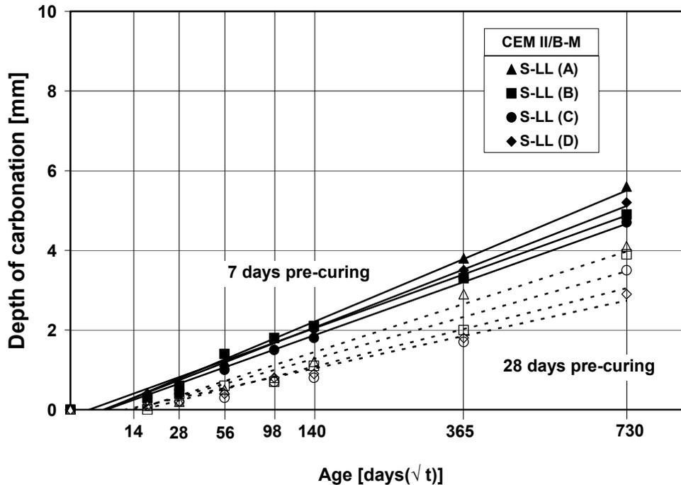
**Figure 3:** Carbonation of mortar prisms stored in laboratory climate 20°C/65% relative humidity with different pre-curing periods (concrete. max. aggregate size 8 mm; cement content 500 kg/m<sup>3</sup>, w/c = 0.50)
