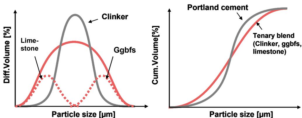
**Figure 1:** Principle changes in particle size distribution of an interground ternary blend
