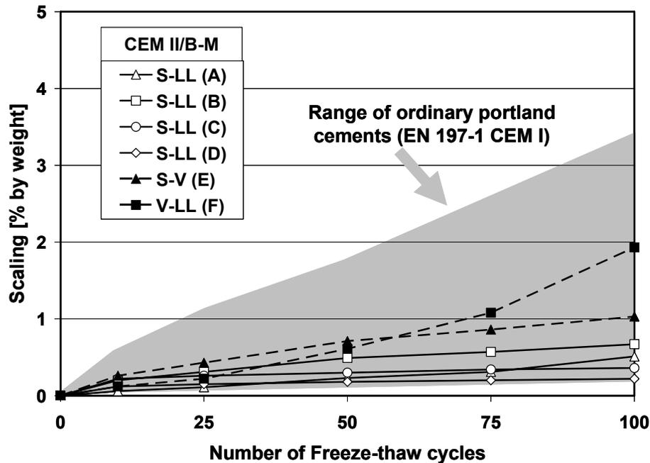
**Figure 5:** Development of scaling of concretes exposed to freeze-thaw cycles (concrete composition: cement content 300 kg/m<sup>3</sup>, w/c = 0.60, no air entrainment)
