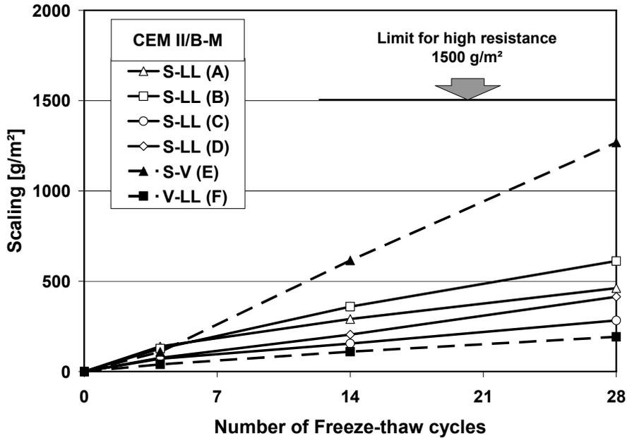
**Figure 6:** Development of scaling of concretes exposed to freeze-thaw cycles and de-icing salts (concrete composition: cement content 320 kg/m<sup>3</sup>, w/c = 0.50, 4.5 % air entrainment)
