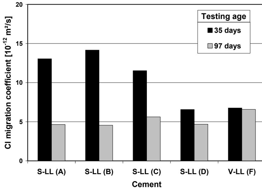
**Figure 4:** Results of Rapid Chloride Migration Test of samples tested at age of 35 and 97 days respectively (concrete composition: cement content 320 kg/m<sup>3</sup>, w/c = 0.50)
