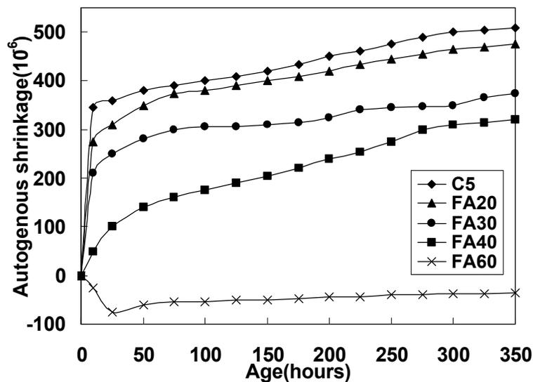
Fig. 3 Effect of fly ash content on autogenous shrinkage of concrete with w/b of 0.25
