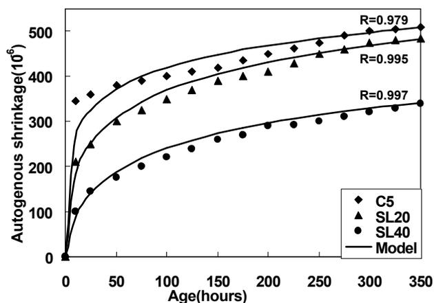
Fig. 6 autogenous shrinkage curves of concretes containing GGBS with  $w/b$  of 0.25 gotten by numerical model and measurement results
