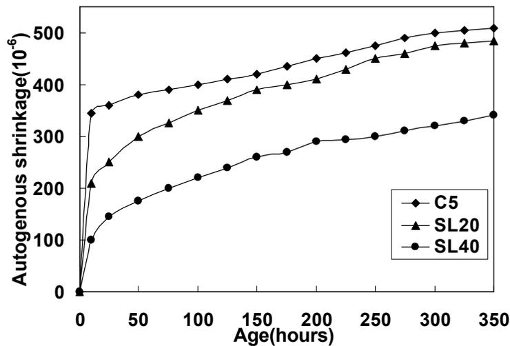
Fig. 4 Effect of GGBS content on autogenous shrinkage of concrete with w/b of 0.25
