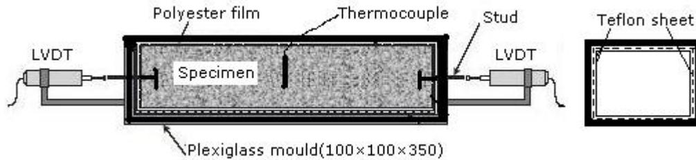
Fig.1 Experimental setup for the measurement of autogenous shrinkage of concrete
