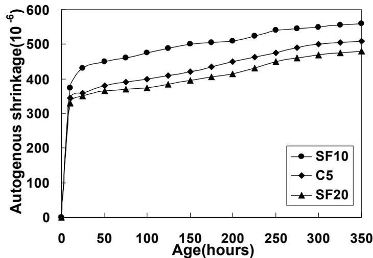
Fig. 5 Effect of silica fume content on autogenous shrinkage of concrete with w/b of 0.25
