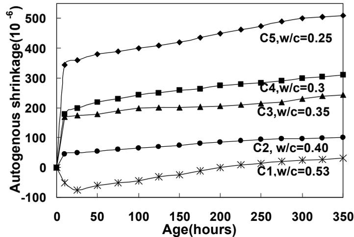
Fig. 2 Effect of w/cm on autogenous shrinkage for concrete prepared with pure Portland cement
