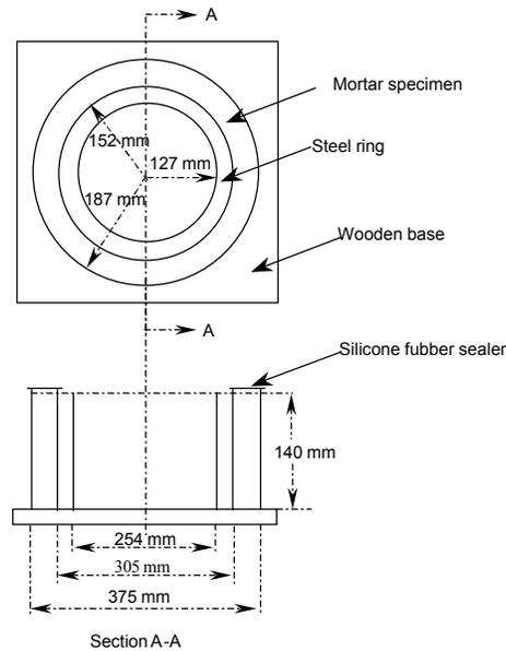
Fig. 3 Test specimen dimensions [13]
