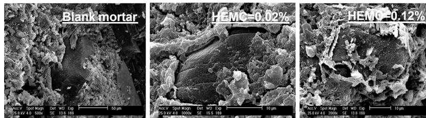
Fig. 5 Structure of cement mortars with HEMC
