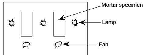
Fig.2 Set-up for the plastic shrinkage cracking test [12]
