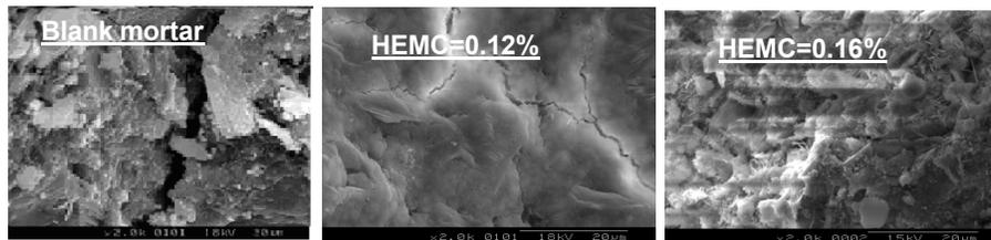
Fig. 6 Slots structure of cement mortars with HEMC
