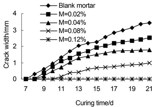
Fig.4 Drying shrinkage cracking width of cement mortars with M
