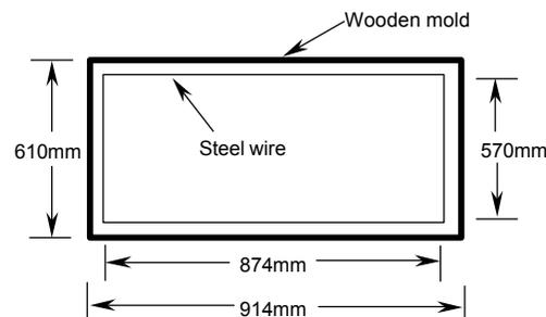
Fig. 1 Schematic of the plastic shrinkage cracking mold [12]
