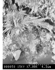
Figure. 7 – Micrograph of OPC cured for 20 years
